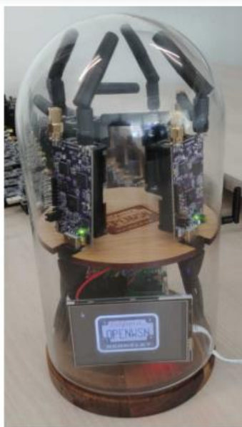
Slika 3.8 OtBox: Raspberry Pi, 4 OpenMote B, ekran i QR kod u staklenom zvonu
